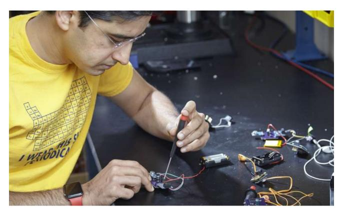
Georgia Tech assistant professor M. Saad Bhamla assembles a prototype LoCHAid, an ultra-low-cost hearing aid built with a 3D-printed case and components that cost less than a dollar. Credit: Craig Bromley
